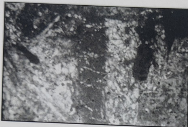
Fig. 6. Highly mechanically fractured and chemically altered plagioclase in gabbro showing diminishing cores of unaltered material ((BCN, 6.3X). Note: Totally altered plagioclase and pyroxene grains.
