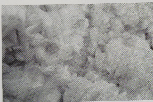
Fig.21. Growth of sheaf-like aggregates of well-developed zeolite crystals
