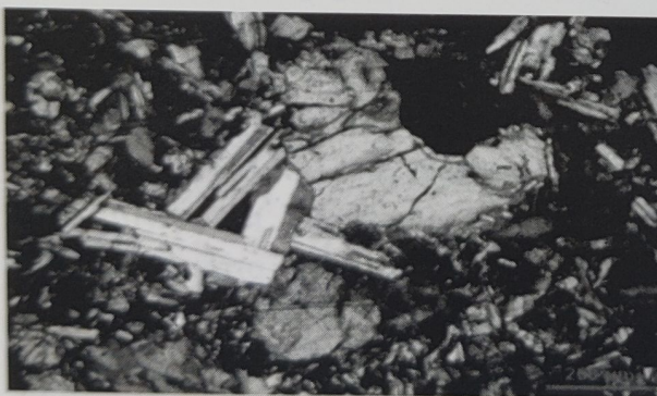
Fig. 8. Porphyritic texture showing the phenocrysts of plagioclase feldspar and pyroxene as well in the groundmass of non-vesicular basalt. (BH2/8)
